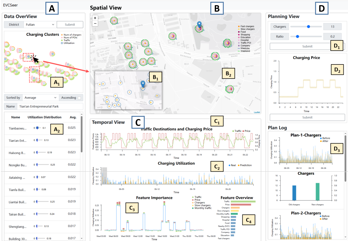
FIGURE 1. Our visualization system, EVCSeer , supports evaluating charging station operations and exploring charging station utilization. The data overview (A) shows an overview of charging stations, including charging clusters and utilization distribution. The spatial view (B) shows the spatial distribution of charging stations and detailed information with glyphs. The temporal view (C) provides temporal information of charging stations and prediction of utilization, as well as exploration of feature importance. The planning view (D) provides “what-if” analysis, where users can adjust different factors and compare corresponding results.
