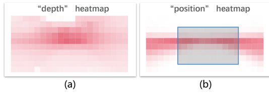
Figure 7: (a) shows car distribution in the “depth” heatmap, while (b) shifts focus to the “position” heatmap for car placement. The manually selected range is highlighted in blue.
